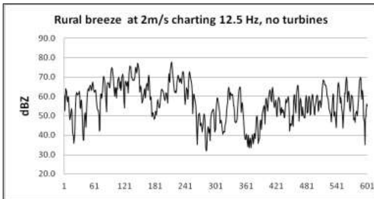
Figure 4.5.3: Outdoor rural natural sound levels in the 12.5Hz LZe q third octave band
