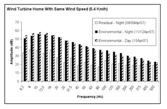
Figure 1. Comparison of ILFN levels in 1/3 octave bands, in dBL, *at the same windspeed*, and recorded inside the master bedroom. Residual (no IWT blade movement); Environmental (with rotating IWT blades) [13].
